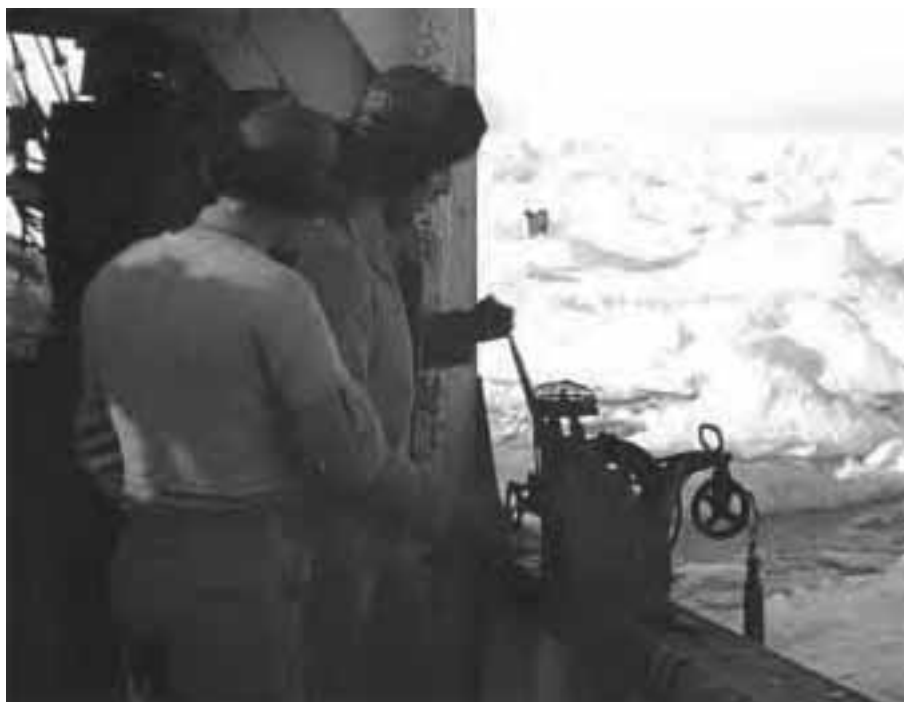
Fig. 36. Urbano and Albertini retract the sounding probe after having measured the sea depth under the drifting Heimen-SUCAI
