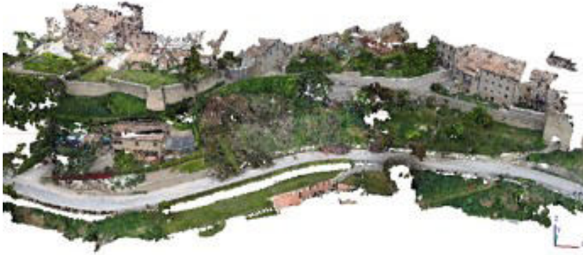
Figure 7.8: Result of the combined point clouds
