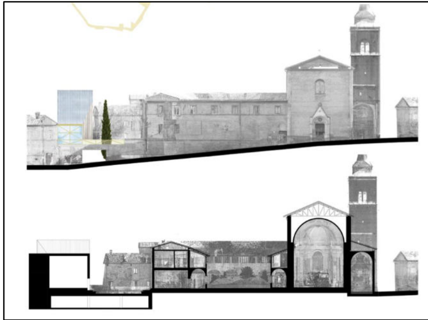
Figure 12.8: Amandola, San Francesco monastery: main facade and section with the post-earthquake damages
