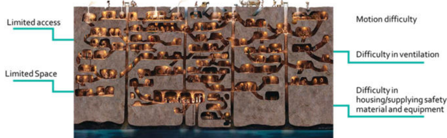
Figure 8.1: General limitations encountered in underground structures
