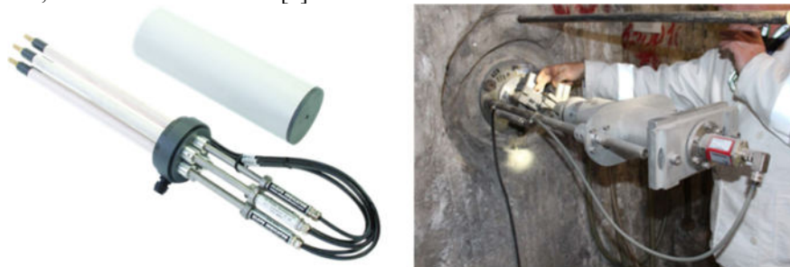
Figure 8.8: Rod Extensometer and its installation [7]
